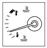
This gage shows the engine coolant temperature.
